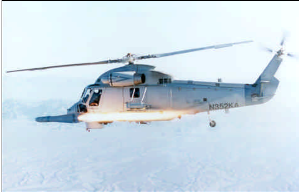
Royal New Zealand Navy SH-2G(NZ) shown during Maverick Missile firing and self-protection system tests at Yuma Proving Grounds, December 2000.
